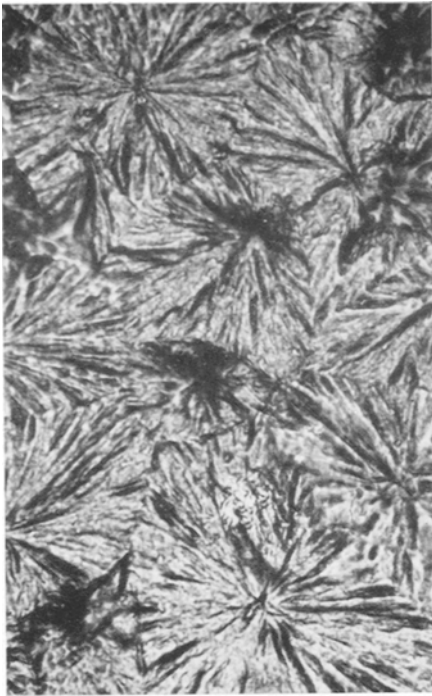
Figure 3 Polypropylene surface after etching for 96 h. The spherulitic microstructure is now fully revealed (reflected light \times 700 ).
